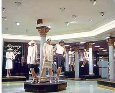
Semi-recessed accent lights are used in retail to focus light on merchandise. These can be repositioned as displays change.
