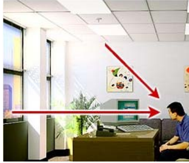
Direct glare from windows and luminaires
